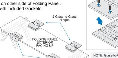
NOTE: Glass-to-Glass Hinge Clamping Plate and Gaskets installed on Folding Panel only.
