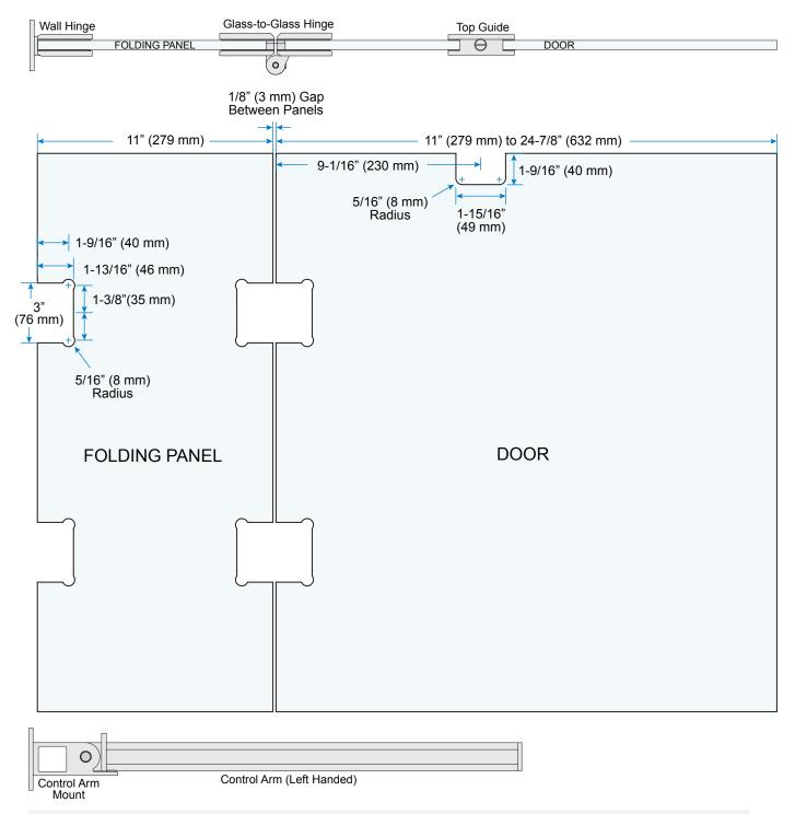
NOTE: For use with 3/8" or 1/2" (10 or 12 mm) Tempered Glass only. Do Not use Laminated Glass.
