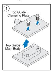
NOTE: Top Guide is installed with Clamping Plate on interior of Door. Glass-to-Glass Door Hinges are installed with Clamping Plates on interior during installation on Page 7.
