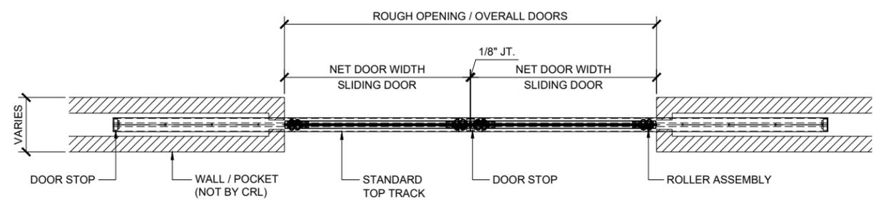
PLAN VIEW - STACKING PARTITION SYSTEM W/DOORS CLOSED (PARKING TYPE 5)
