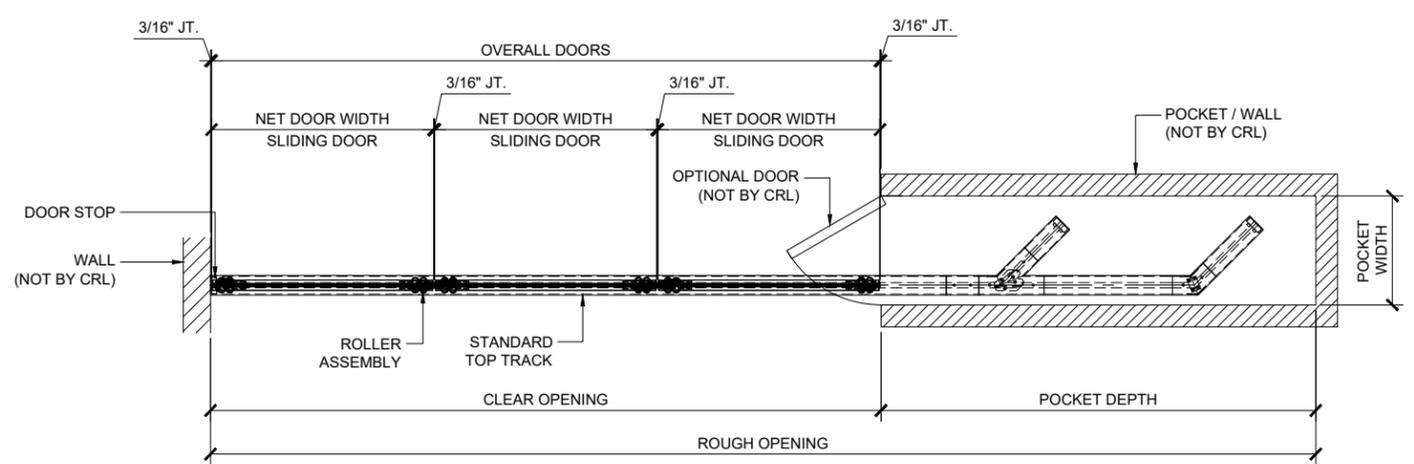
PLAN VIEW - TYP. STACKING PARTITION SYSTEM W/DOORS CLOSED (PARKING TYPE 3)
