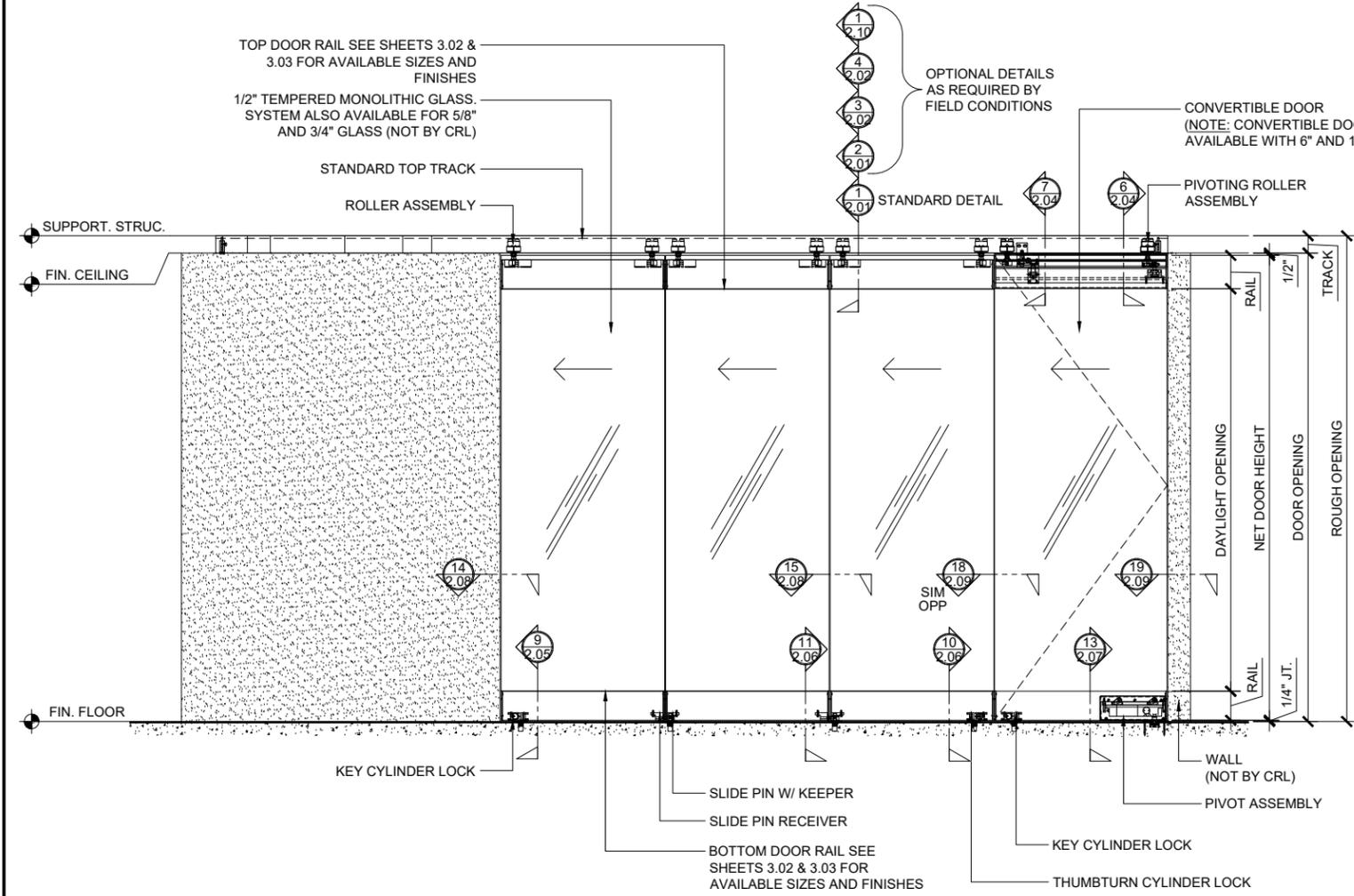
ELEVATION - STACKING PARTITION SYSTEM W/DOORS (PARKING TYPE 2)
