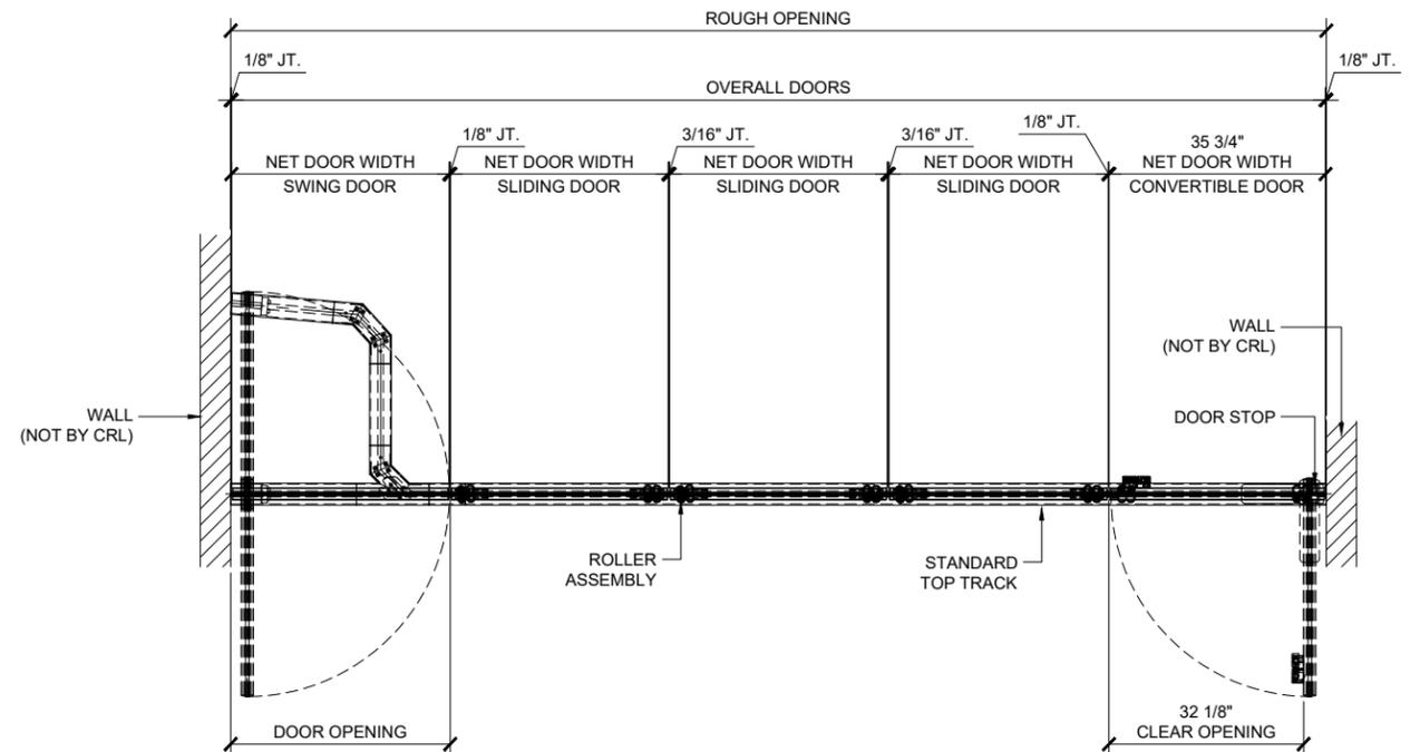
PLAN VIEW - STACKING PARTITION SYSTEM W/DOORS CLOSED (PARKING TYPE 1)
