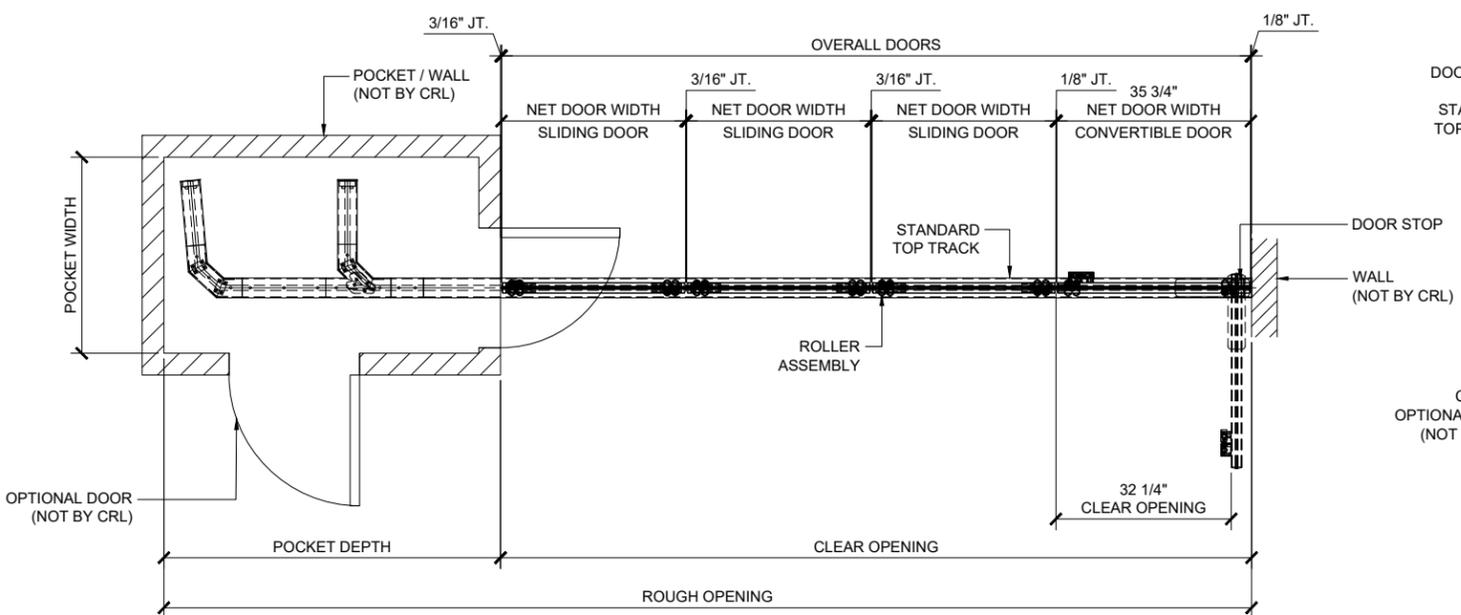
PLAN VIEW - STACKING PARTITION SYSTEM W/DOORS - DOORS CLOSED (PARKING TYPE 2)
