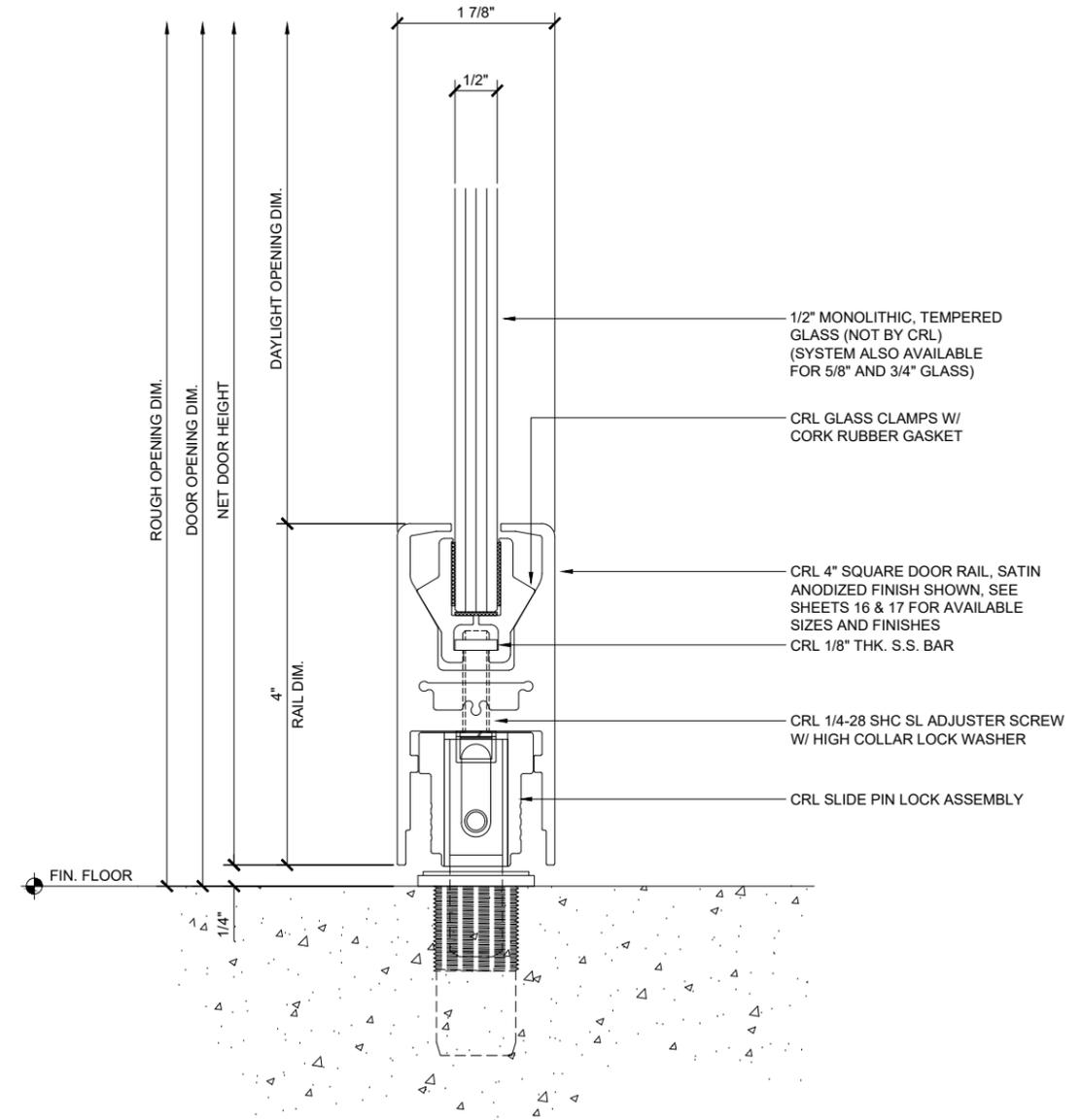
11 DOOR HEAD - AT SLIDE PIN LOCK ASSEMBLY
