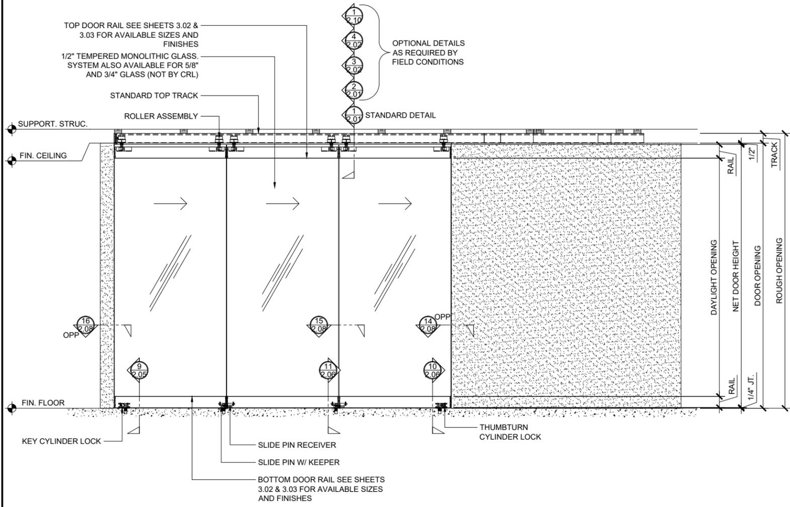
ELEVATION - TYP. STACKING PARTITION (PARKING TYPE 3)
