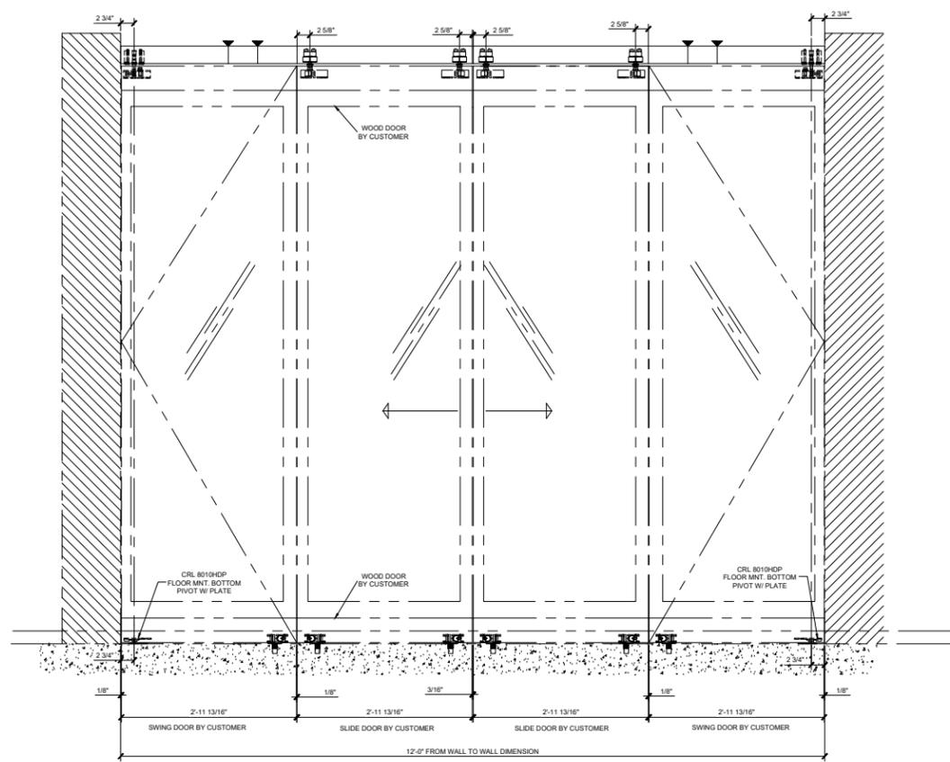
ELEVATION - TYP. STACKING PARTITION SYSTEM (PARKING TYPE 4)
