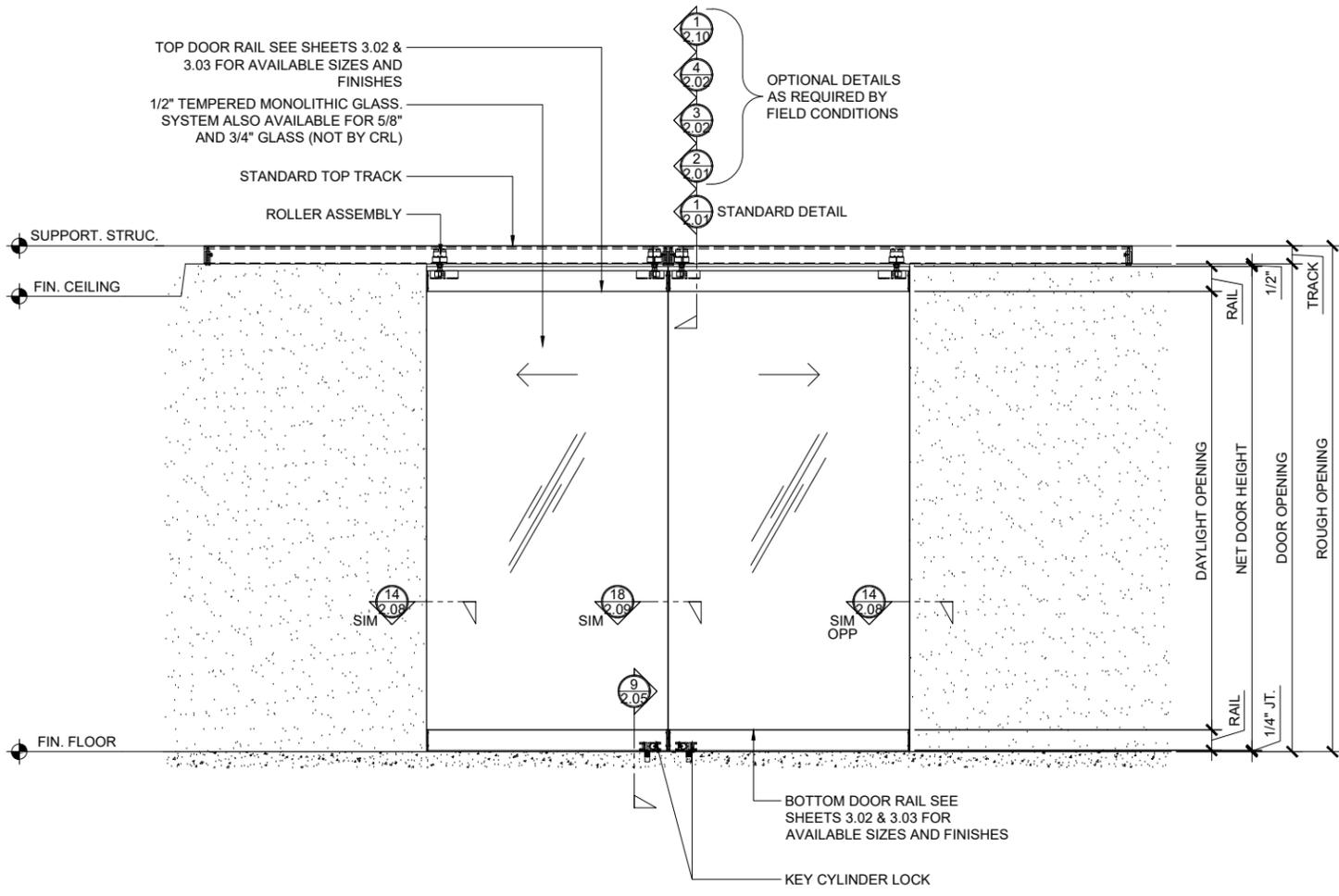
ELEVATION - STACKING PARTITION SYSTEM (PARKING TYPE 5)
