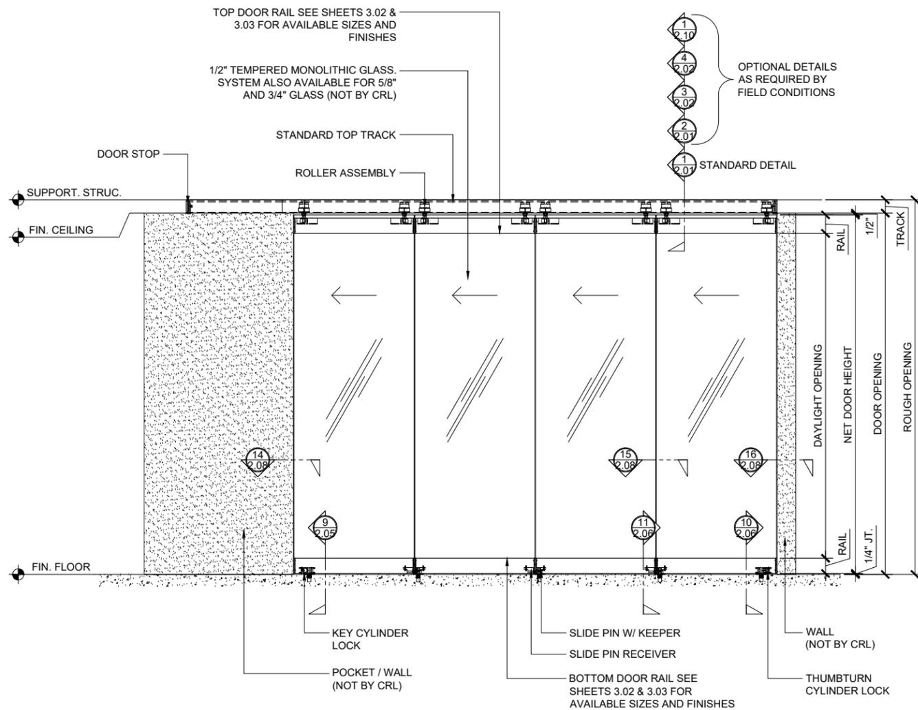
ELEVATION - TYP. STACKING PARTITION SYSTEM (PARKING TYPE 1)
