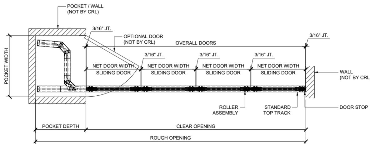
PLAN VIEW - TYP. STACKING (DOOR CLOSED PARKING TYPE 1)
