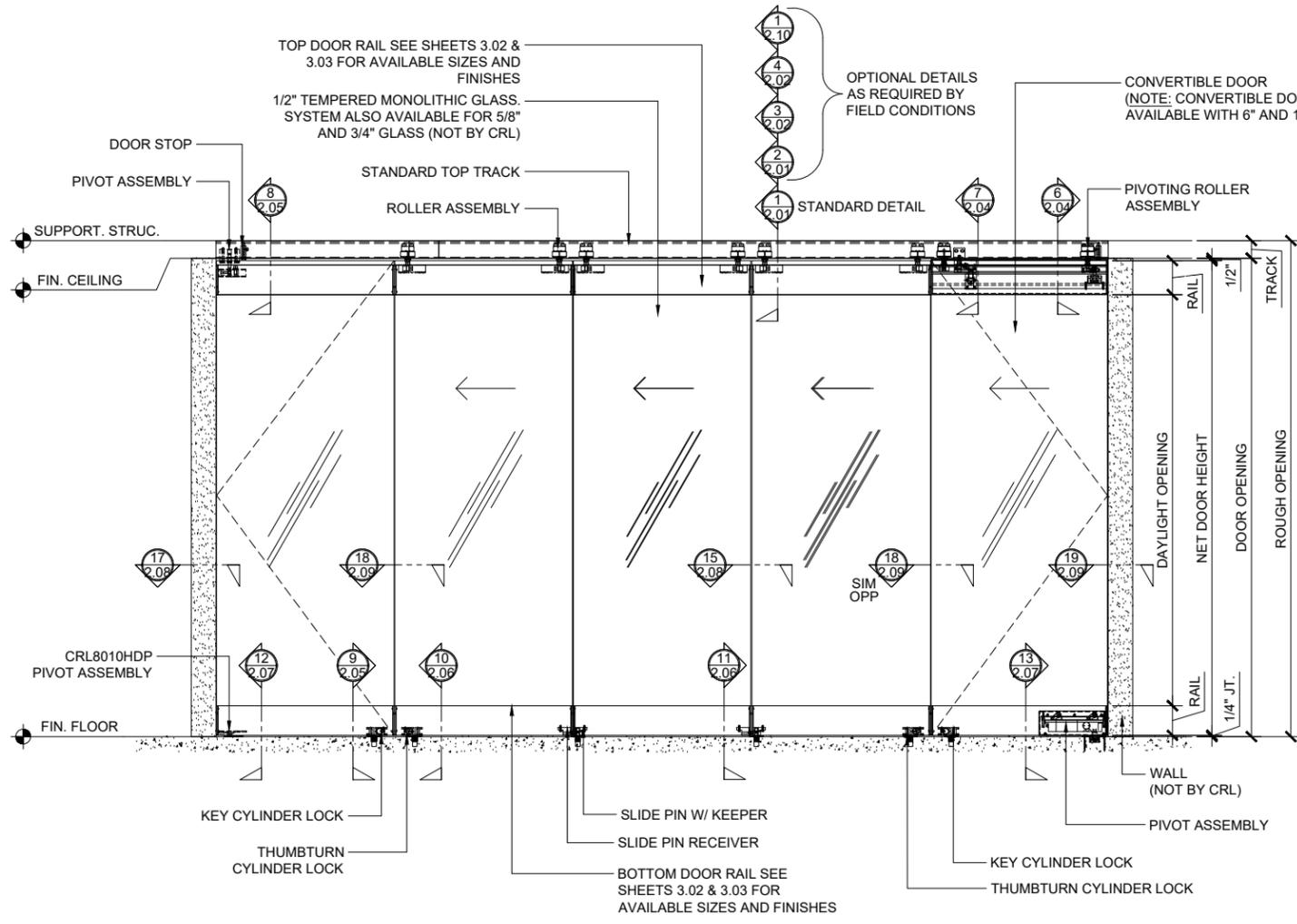
ELEVATION - STACKING PARTITION SYSTE, W/DOORS (PARKING TYPE 1)
