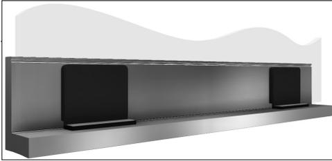
Make sure the TAPER-LOC® spacing does not exceed 14" (356 mm) on center.
